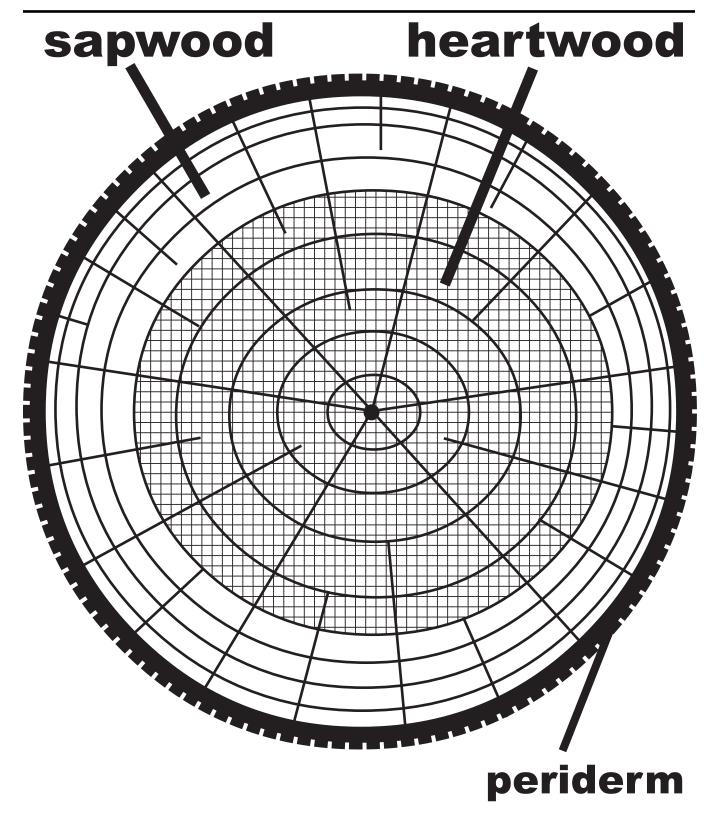
Figure 11: Diagram of a tree stem cross-section showing sapwood and heartwood (shaded).
