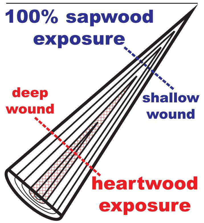
Figure 12: Diagram of a deep cut and a shallow cut using heartwood exposure to gauge relative wound depth.
