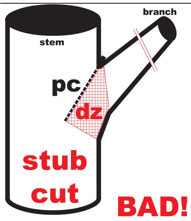
Figure 6: Diagram of stem - branch confluence area with an abusive, improper stub cut applied.
